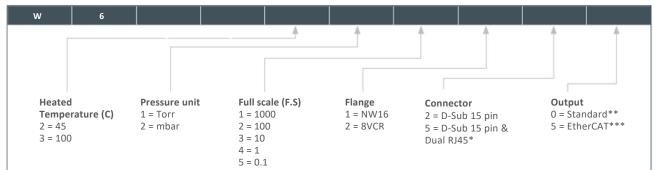
\*Only selectable with pressure units of torr and Output of "EtherCAT".
