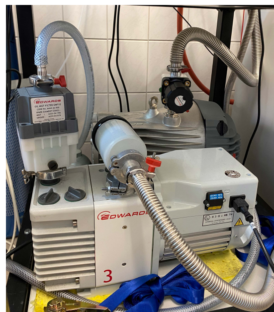
Friedrich Schiller University Jena vacuum pump setup: RV3, nXDS and accessories
