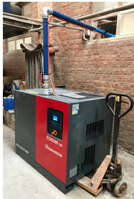
Edwards EOSi oil-injected screw vacuum pump
