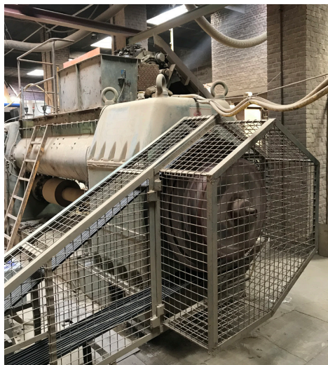
Clay moved into the extrusion machine
