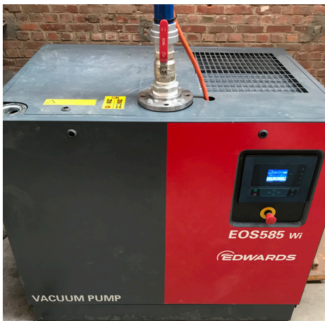
Edwards EOSi oil-injected screw vacuum pump
