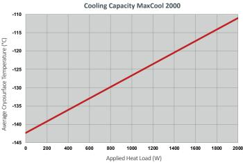
Single-circuit model; temperature shown is average of inlet and outlet temperature using typical cryocoil size; temperature difference between inlet and outlet at maximum load is typically 20°C; end point of curve is maximum load; performance at 50Hz can be  $3-5^{\circ}$ C warmer than 60Hz performance shown;  $25-28^{\circ}$ C cooling water.
