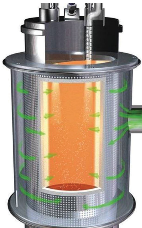
Figure 2. An inward fired combustor maintains uniform temperature and separates fuel gas from process gases to avoid creating PFCs in the abatement process.
