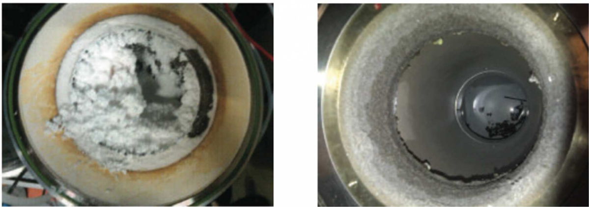
FIGURE 4. An example of continuous improvement and application of best known methods in a point-of-use abatement system: in a TEOS CVD process the standard inward-fired burner (left, after 9k wafers) was replaced with a shortened version (right, after 26k wafers). The resulting increase in surface firing rate greatly reduced unwanted deposition, improving the mean time between service (MTBS) from 10K wafers to 42K wafers.
