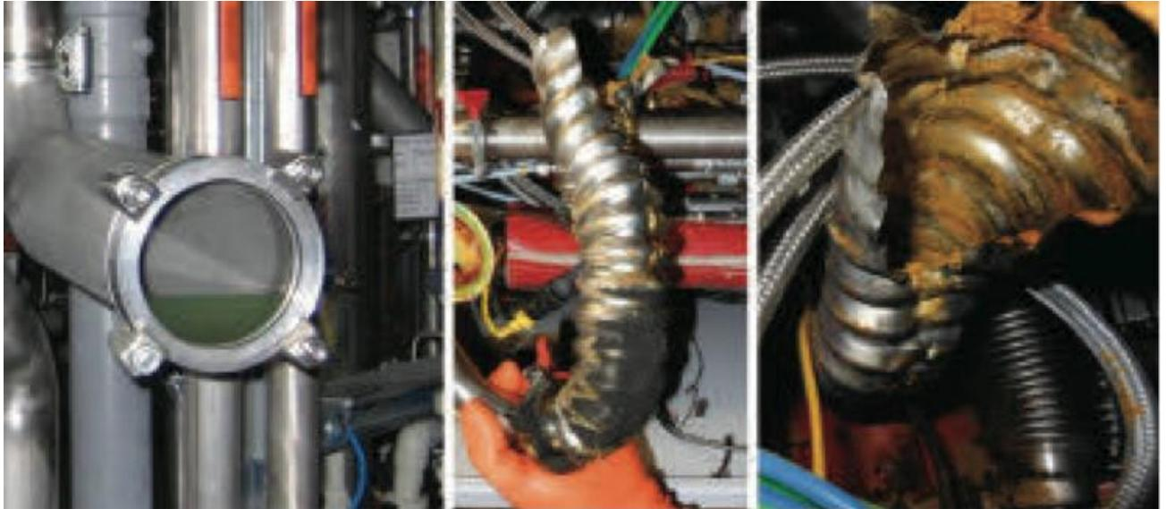
FIGURE 1. (left) Condensed explosive polysiloxane material in an epitaxial deposition system process foreline, (middle and right) CVD exhaust pipe destroyed by explosion of condensed process by-product.
