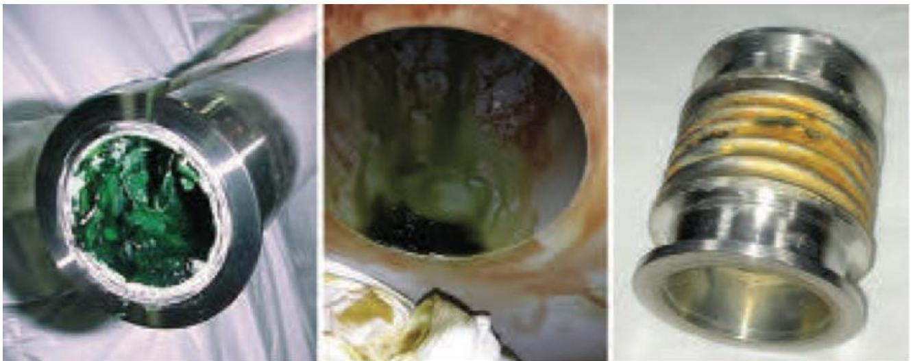
FIGURE 2. (left) Acidic TEOS-based polymer with a pH of approximately 1, (middle) Condensed corrosive Br<sub>2</sub>-based liquid, (right) Exhaust pipe damaged by exposure to condensed acidic material.
