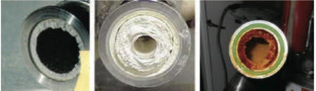
FIGURE 3. Exhaust blockage caused by various materials (left)  $\text{AlCl}_3$  from a metal etch process, (middle)  $\text{NH}_4\text{Cl}$  from an LPCVD process, (right) Unknown material deposited in the exhaust of a metal carbide CVD process.
