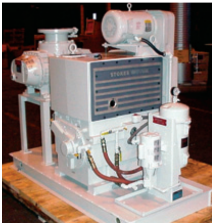
Fig. 1. Oil sealed piston pump with mechanical booster and oil purifier
