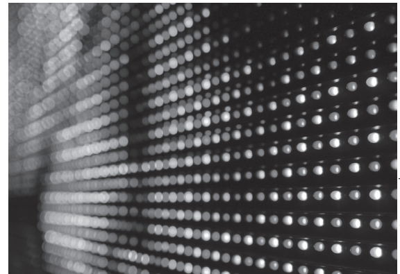
Red, green, and blue LEDs (the “primary colors”) are increasingly being used to provide the background illumination for flat-panel displays, replacing traditionally-used CCL lamps. A big driver is for flat panel TV, where the much better “color gamut” means that colors on screen are closer to the originals. Other advantages for laptop computer applications are thinner screens, reduced weight and longer battery life.
