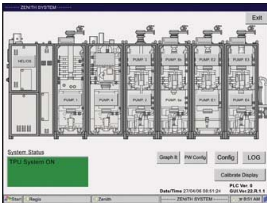
Figure 5. Edwards Zenith™ line of integrated vacuum and abatement systems provides a single user friendly control and monitoring interface for all components.
