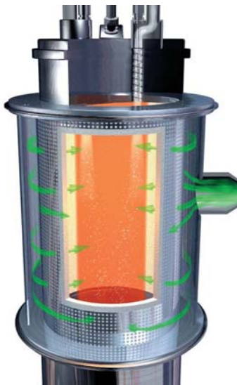
Figure 4. With the inward fired combustor design, the heating fuel gases remain outside the interior reaction chamber. This significantly improves the ability to control temperature compared to open flame systems, thereby improving abatement performance.
