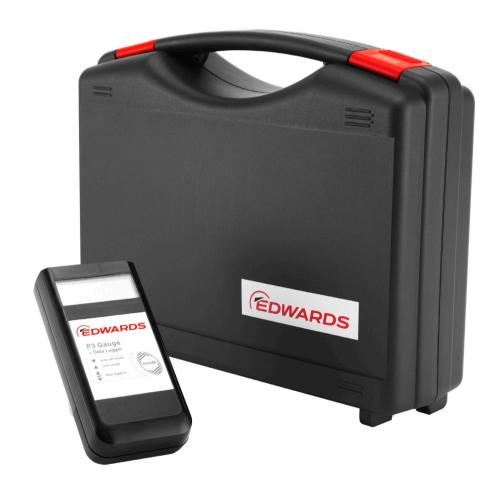
The Edwards P3 handheld measuring system is the essential device for on-site service calls and on the spot flexible checking. Thanks to the easy use and integrated measurement data memory, pressures can be directly measured at different locations for monitoring the application. Owing to the advanced measuring range of the high-precision Piezo/Pirani sensor, pressure measurement in the range of  $1200 \text{ to } 5x10^{-4} \text{ mbar can be displayed.}$
