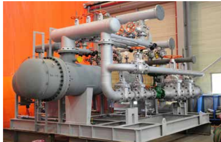
Steam ejector condenser package
