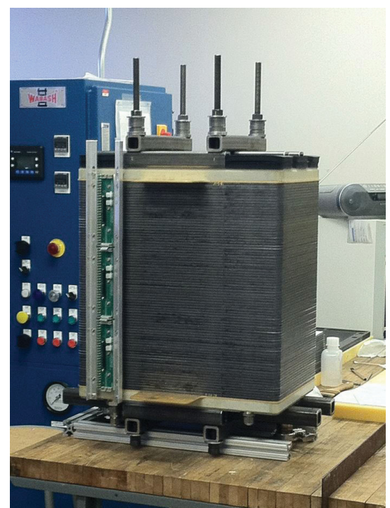
Figure 1. (left) operating principles of the electrochemical cell and (right) a stack of cells assembled to handle larger gas flow.
