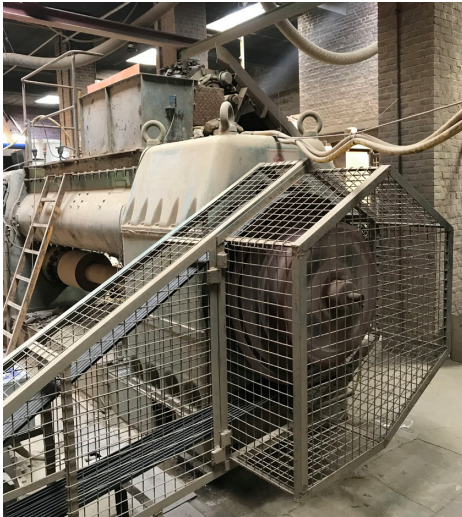
Clay moved into the extrusion machine
